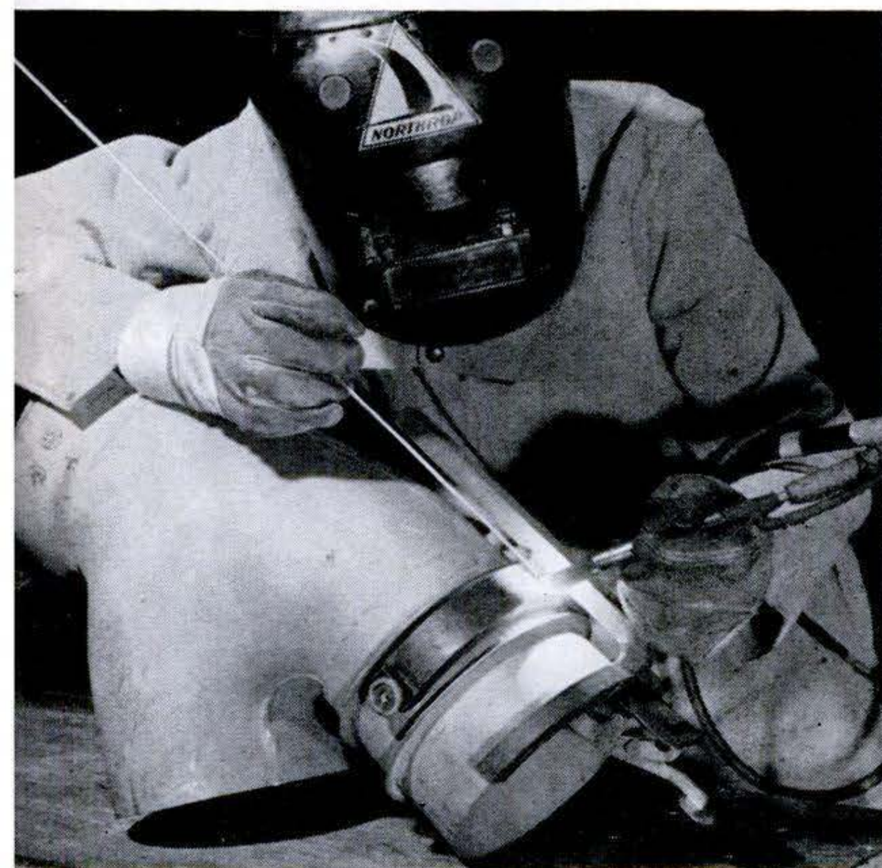
MAGNESIUM requires no flux when welded by Northrop's Heliarc process (above). Helium or argon gas from tube (at right) bathes arc and weld areas, keeps air from molten weld.
